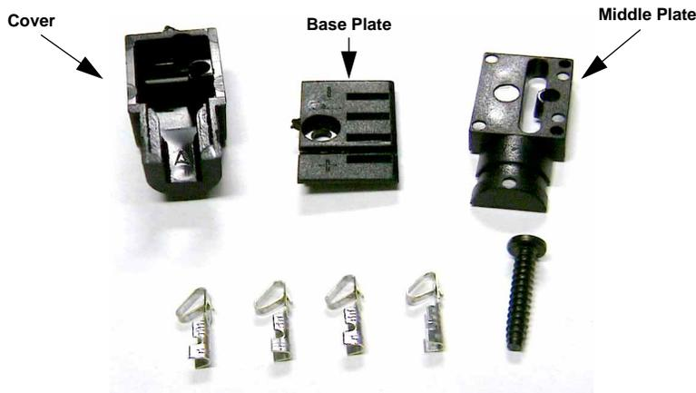
The first step in assembling the connector is to bend the four spring clips at right angles as indicated in the picture to the left. If you want, you can use needlenose pliers, but be careful that you do not accidentally compress either the end of the pins that the wires will be soldered to, or the spring clips themselves.
