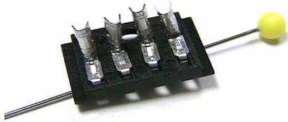
Now, you can pass wires in your cable through the slot in the middle plate, and solder them to
